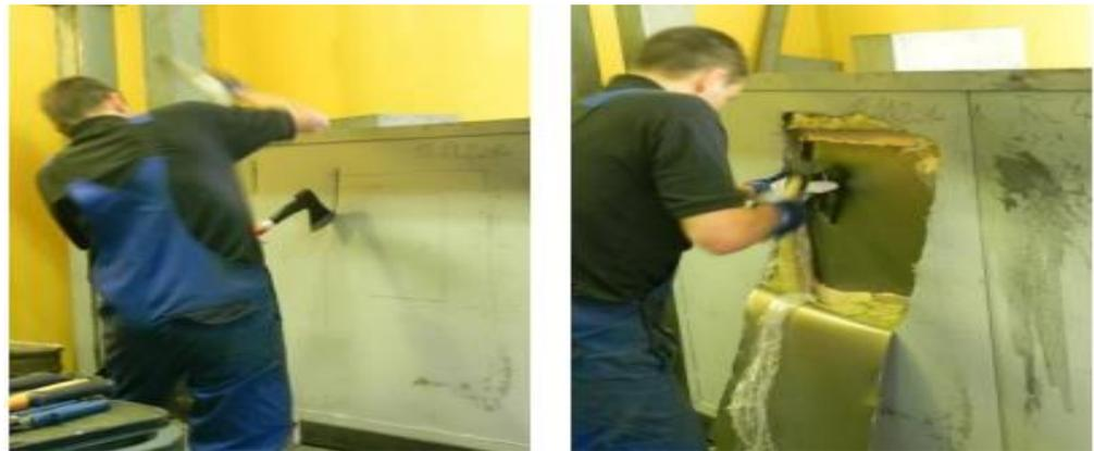
**Figure 1.** 4th Resistance Class panel walls break-through testing [17].
