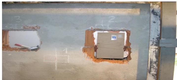
**Figure 2.** Breaking test of masonry made of ceramic blocks [18].
