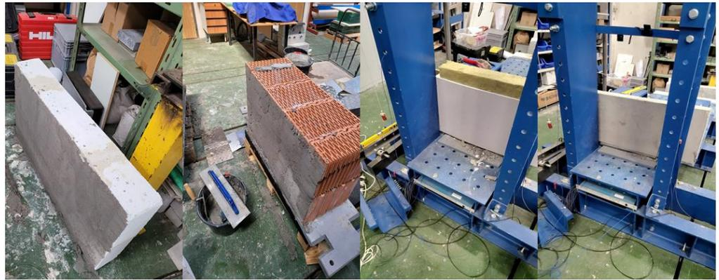
**Figure 3.** Testing samples, from the left—aerated concrete, ceramic brick, plasterboard, reinforced concrete.
