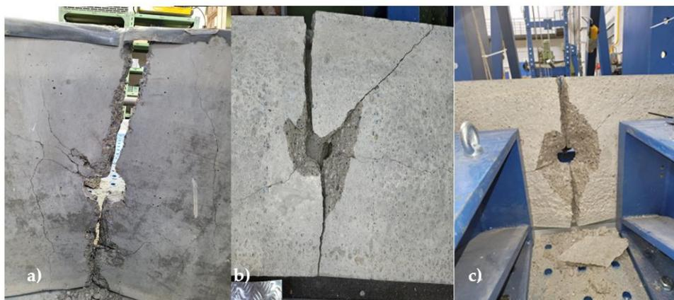
**Figure 9.** Results of reinforced concrete—(a) gradual increase method, (b) maximum height method, (c) constant height method.
