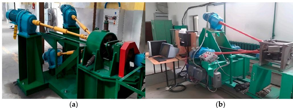
**Figure 1.** The used radial shear rolling mills (a) RSP-14/40 (PCz, Poland); (b) RSP-10/30 (KSU, Kazakhstan).
