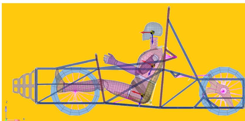
**Figure 1.** Dummy equipped with belt and impact attenuator.
