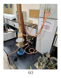
**Figure 3.** Tests conducted on the hardened pervious concrete: (**a**) axial compression; (**b**) split tensile; (**c**) permeability.
