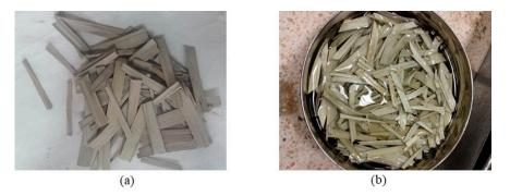
Figure 2. Local date palm leaves fibers used in the study: (a) dry; (b) soaked.
