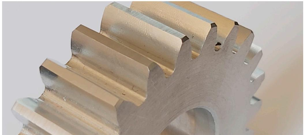
**Figure 13.** Tool paths after multipass machining of gear with longitudinal tooth modification.
