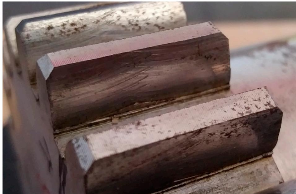
**Figure 12.** Traces of machining using the InvoMilling method.
