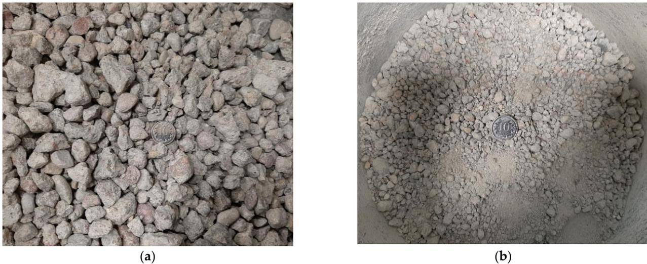
**Figure 2.** View of tested RCA: (a) raw crushed concrete; (b) prepared final mixture.
