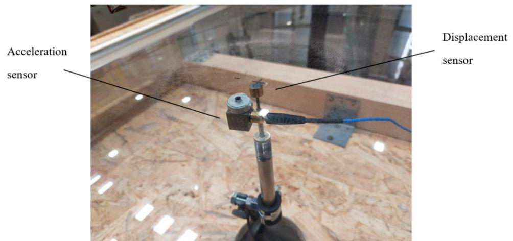
**Figure 5.** Sensors attached to the sample.
