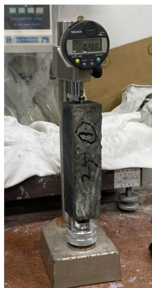
Figure 8. Testing drying shrinkage.
