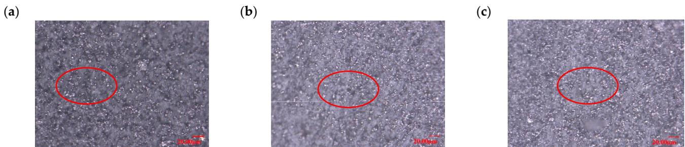
**Figure 3.** Cross-section microscopic morphology of isotropic MRE with 60% mass fraction at different ratios of hybrid size CIPs (CD:CN): (a) 1:3; (b) 1:1; and (c) 3:1.
