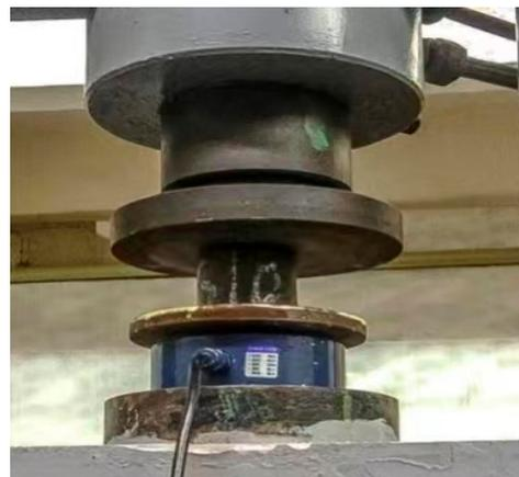
**Figure 2.** Unconfined compressive strength test.
