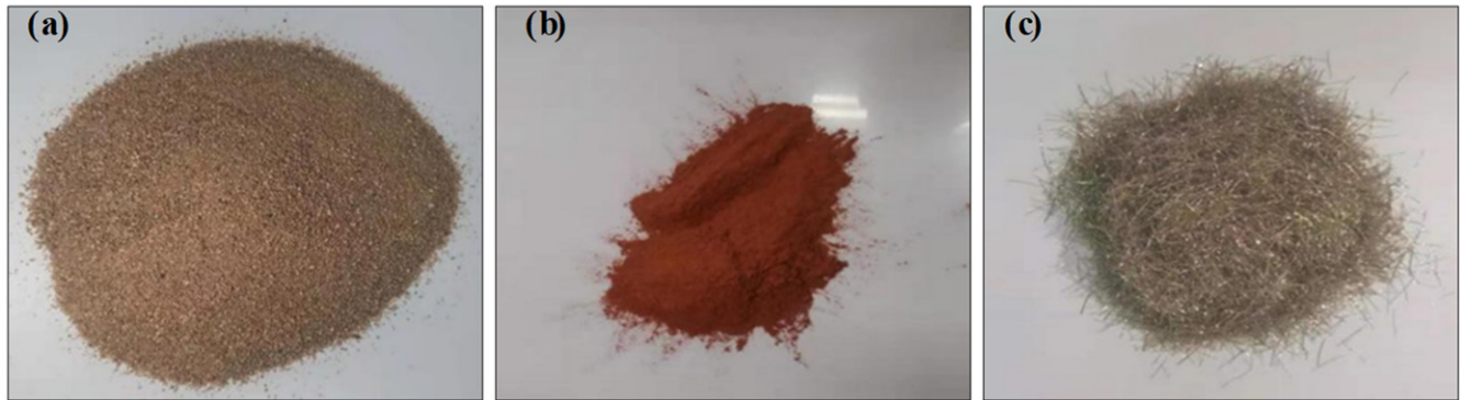
Figure 1. Raw materials used in UHPC: (a) river sand; (b) recycled brick powder; (c) steel fiber.
