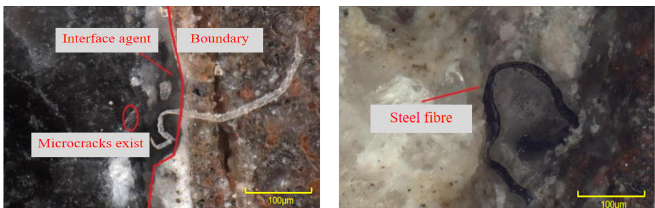
Figure 17. The UHPC-NC bonding interface was magnified 500 times after applying the interface agent.
