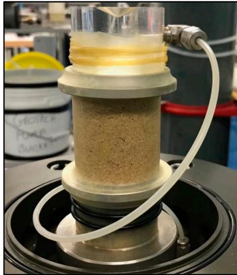
**Figure 3.** The sample positioned in the triaxial cell with enlarged and lubricated end platens.
