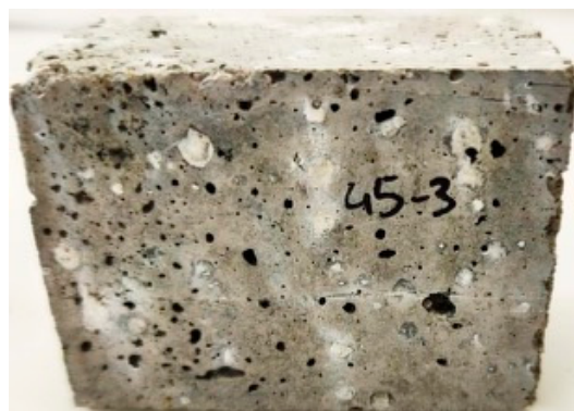
Figure 11. Efflorescence is present on the surface of the mortar A 50 .
