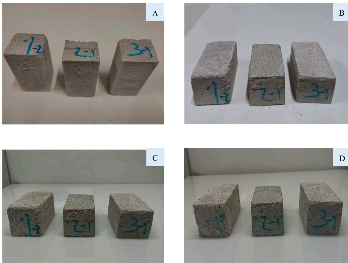
Figure 15. Mortars appearance after (A) 0 cycles (28 days of curing), (B) 5 cycles, (C) 15 cycles, and (D) 25 cycles (1—B 0 , 2—B 15 , and 3—F 5–63 ).
