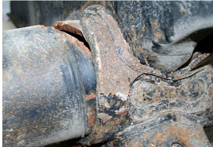
**Figure 14.** Axis fracture location.
