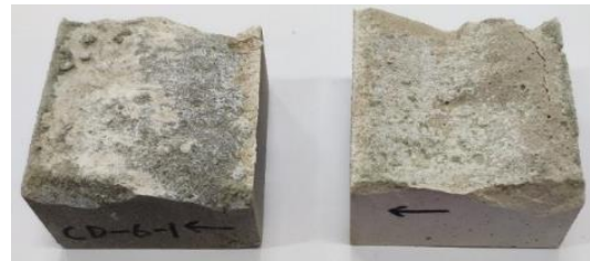
Figure 14. Failure surfaces of CD-3 after the first shearing.
