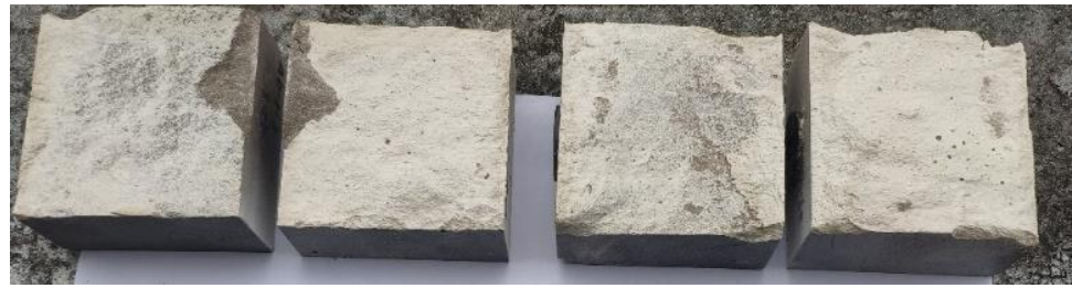
Figure 13. Failure surfaces of AD-1 and AD-2 after the first shearing.
