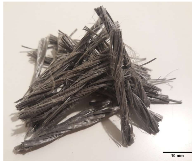
Figure 1. Twisted fibers used in the manufacturing of fiber-reinforced concrete.
