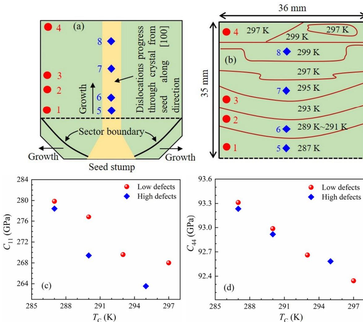
**Figure 9.** Schematic illustration of (a) spatial heterogeneity and (b) spatial dependence of  $T_C$  in a composition gradient on Li-doped KTN wafer. Diamonds (blue) and closed circles (red) denote the regions with high and low defect density, respectively. The elastic constants (c)  $C_{11}$  and (d)  $C_{44}$  of a composition gradient Li-doped KTN wafer as a function of position. The data were adapted from Refs. [58,111].
