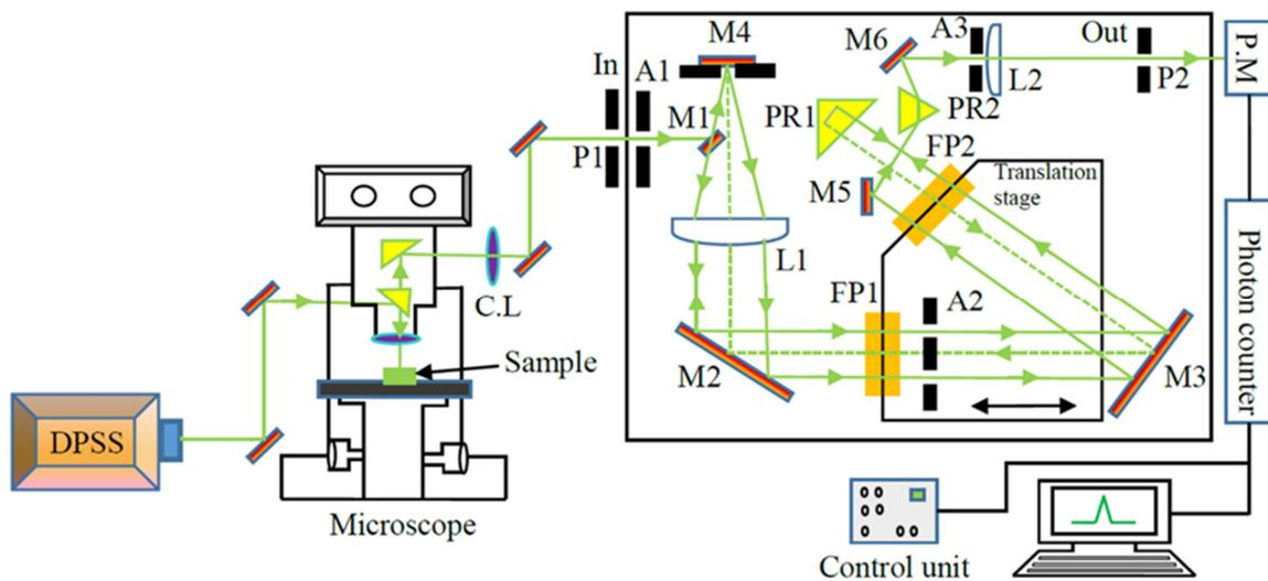
**Figure 1.** A schematic illustration of a Sandercock 3 + 3 pass tandem interferometer equipped with a photomultiplier and optical microscope [57,58].
