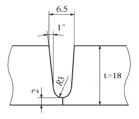
Figure 3. Schematic diagram of the ultra-NGMAGW welding groove.
