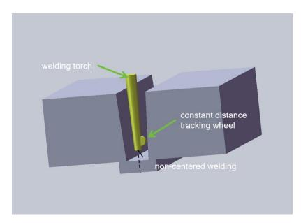
Figure 2. Schematic diagram of the ultra-NGMAGW device.
