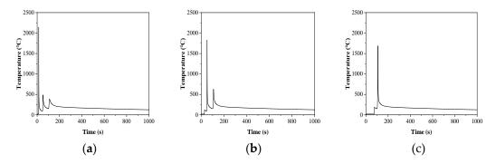
**Figure 18.** Welding thermal simulation of thermal cycle curve in the weld zone: (**a**) the first weld; (**b**) second weld; and (**c**) third weld.
