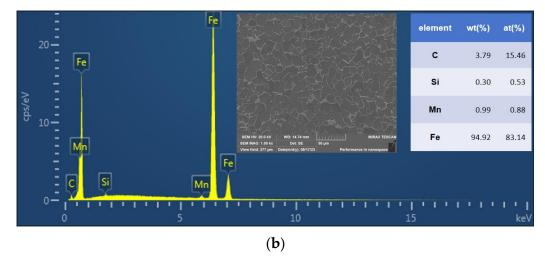
**Figure 16.** (**a**) EDS spectrum for the ultra-NGMAGW welded joints, and (**b**) EDS spectrum for the NGSAW welded joints.
