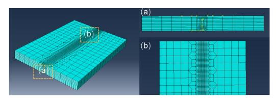
Figure 5. Q235A thick plate joint finite element model. (a) weld cross-section; (b) weld surface.
