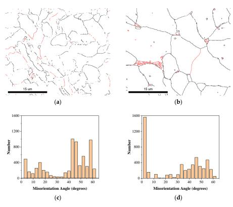
**Figure 14.** Adjacent grain boundary misorientation distribution map and angle statistical map at the WZ: (**a**) adjacent grain boundary misorientation distribution map of ultra-NGMAGW joint; (**b**) adjacent grain boundary misorientation distribution map of the NGSAW; (**c**) angle statistical map of the ultra-NGMAGW; and (**d**) angle statistical map of the NGSAW.
