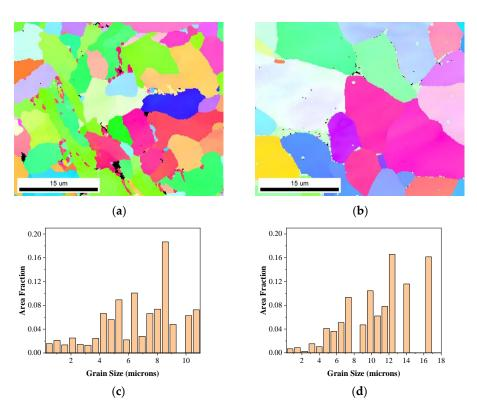
**Figure 13.** Inverse pole figure and grain size distribution diagram at the WZ: (**a**) inverse pole figure of the ultra-NGMAGW joint; (**b**) inverse pole figure of the NGSAW joint; (**c**) grain size distribution diagram of the ultra-NGMAGW joint; and (**d**) grain size distribution diagram of the NGSAW joint.
