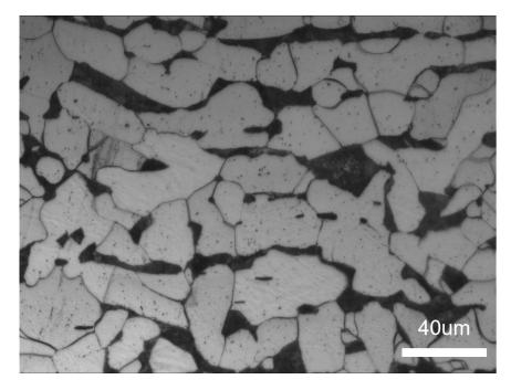
Figure 1. Microstructure of Q235A base metal.
