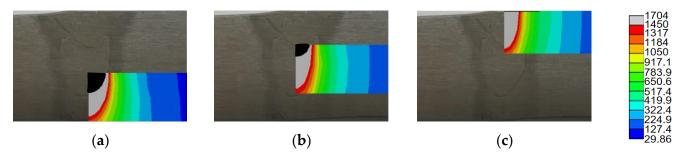
Figure 17. Temperature distribution of welded joint: (a) first weld; (b) second weld; and (c) third weld.
