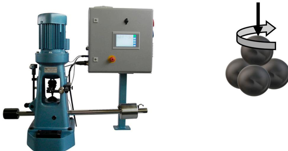
**Figure 1.** Four-ball tester and the principle of measurements.
