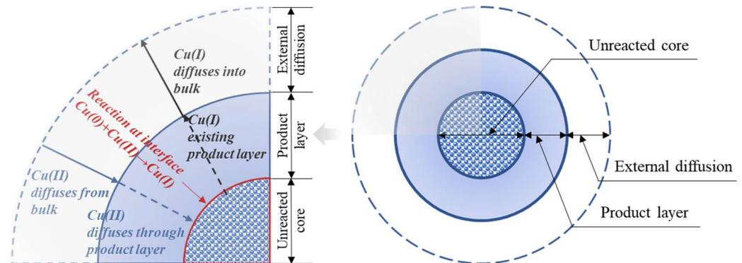
**Figure 2.** Schematic illustration of the mechanism and kinetic considerations in a Cu-ammoniacal leaching system. Adapted from reference [28].
