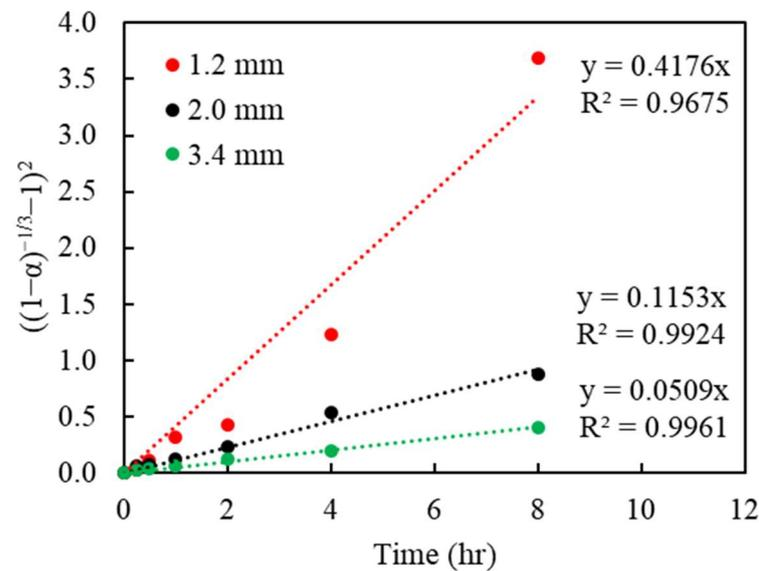
**Figure 7.** Plot of  $\left((1-\alpha)^{-\frac{1}{3}}-1\right)^2$  vs. time under various particle sizes (diameter, mm); the data correspond to those in Figure 4.
