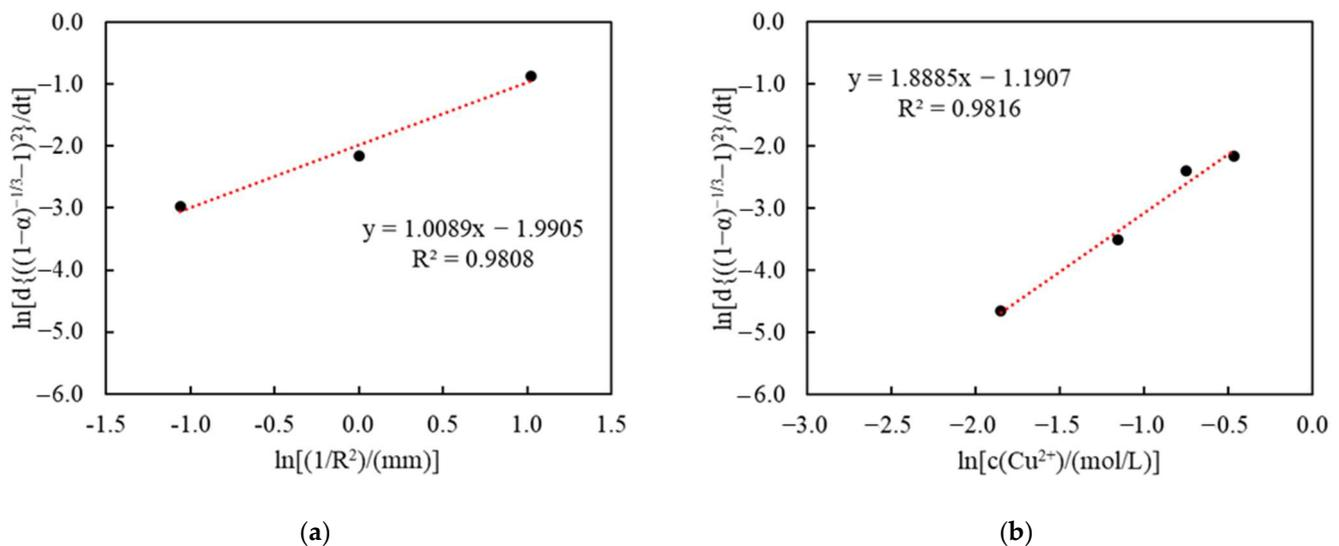
**Figure 10.** Estimation of the reaction order: plot of  $\ln\left[\frac{d}{dt}\left\{\left(1-\alpha\right)^{-1/3}-1\right\}^2\right]$  vs.  $\ln\left[\left(\frac{1}{R^2}\right)/(\text{mm})\right]$  (a), and plot of  $\ln\left[\frac{d}{dt}\left\{\left(1-\alpha\right)^{-1/3}-1\right\}^2\right]$  vs.  $\ln\left[c\left(\text{Cu}^{2+}\right)/(\text{mol/L})\right]$  (b).
