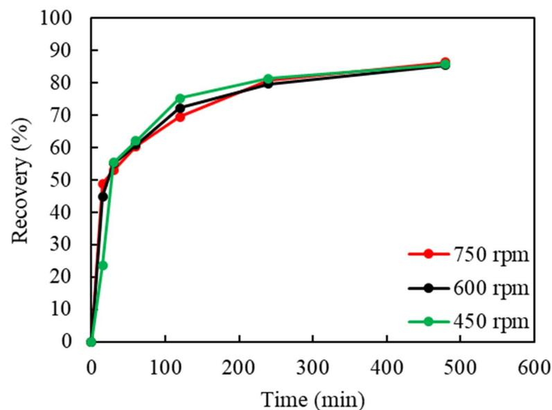
**Figure 3.** The effect of the stirring rate (rpm) on Cu recovery in ammoniacal leaching. (S/L ratio: 50 g/L,  $(\text{NH}_3)_2\text{SO}_4$ : 1 M,  $\text{NH}_4\text{OH}$ : 4 M, Cu(II): 40 g/L, particle size:  $-2$  mm, temp. 18 °C).
