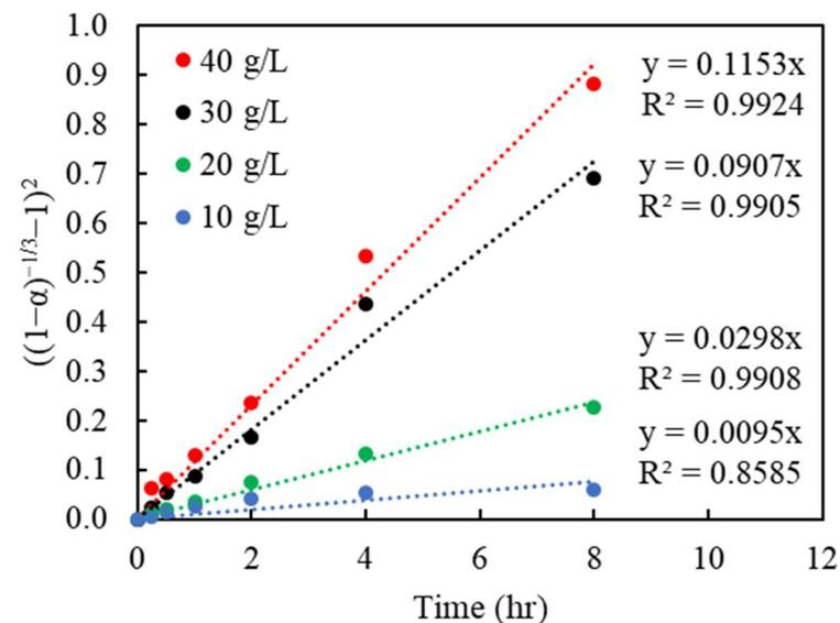
**Figure 8.** Plot of  $\left((1-\alpha)^{-\frac{1}{3}}-1\right)^2$  vs. time under various initial Cu(II) concentrations (g/L); the data correspond to those in Figure 5.
