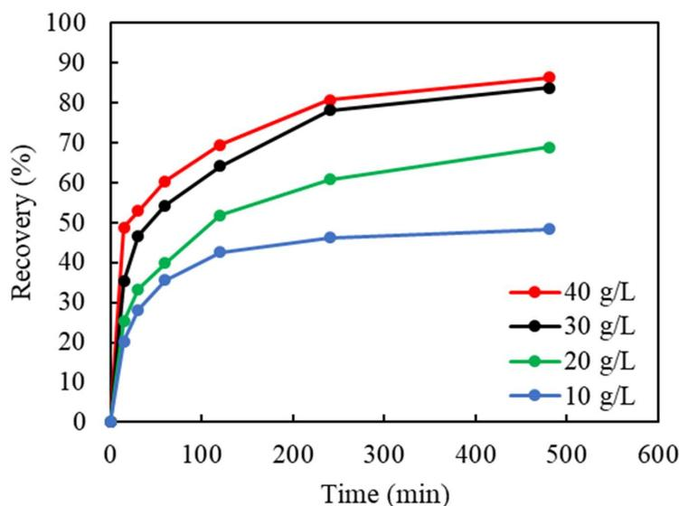
**Figure 5.** The effect of the initial Cu(II) concentration (g/L) on Cu recovery in ammoniacal leaching (S/L ratio: 50 g/L, (NH<sub>3</sub>)<sub>2</sub>SO<sub>4</sub>: 1 M, NH<sub>4</sub>OH: 4 M, particle size: −2 mm, stirring: 750 rpm, temp.: 18 °C).
