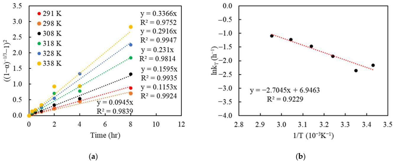
**Figure 9.** Plot of  $\left((1 - \alpha)^{-\frac{1}{3}} - 1\right)^2$  vs. time under various temperatures ( $^{\circ}\text{C}$ ) (a), and the Arrhenius plot for Cu ammoniacal leaching (b); the data correspond to those in Figure 6.
