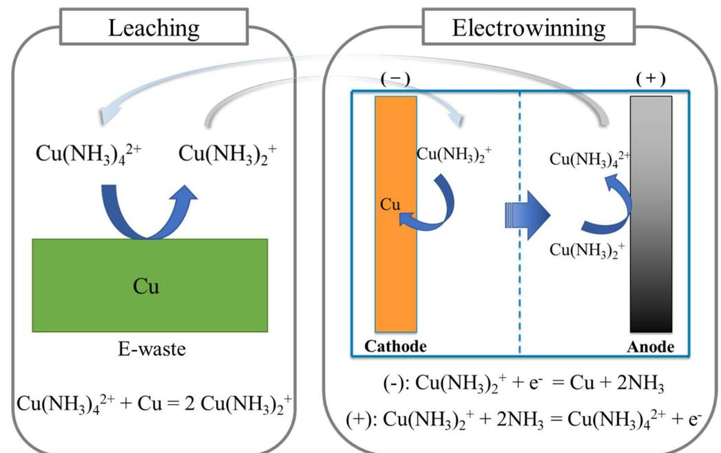
**Figure 1.** Schematic illustration of the coupled leaching-EW circuit in the Cu(II)-NH<sub>3</sub>-SO<sub>4</sub> system. Adapted from references [7,16].
