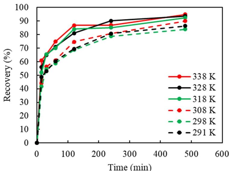
**Figure 6.** The effect of the temperature (°C) on Cu recovery in ammoniacal leaching (S/L ratio: 50 g/L, (NH<sub>3</sub>)<sub>2</sub>SO<sub>4</sub>: 1 M, NH<sub>4</sub>OH: 4 M, Cu(II): 40 g/L, particle size: −2 mm, stirring: 750 rpm).
