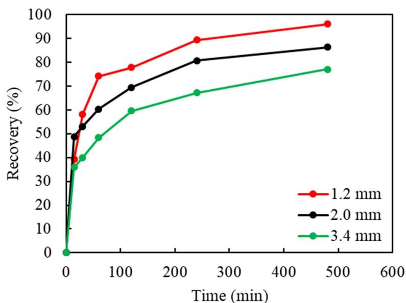
**Figure 4.** The effect of the particle size (top size, diameter, mm) on Cu recovery in ammoniacal leaching (S/L ratio: 50 g/L,  $(\text{NH}_3)_2\text{SO}_4$ : 1 M,  $\text{NH}_4\text{OH}$ : 4 M, Cu(II): 40 g/L, stirring: 750 rpm, temp.: 18 °C).
