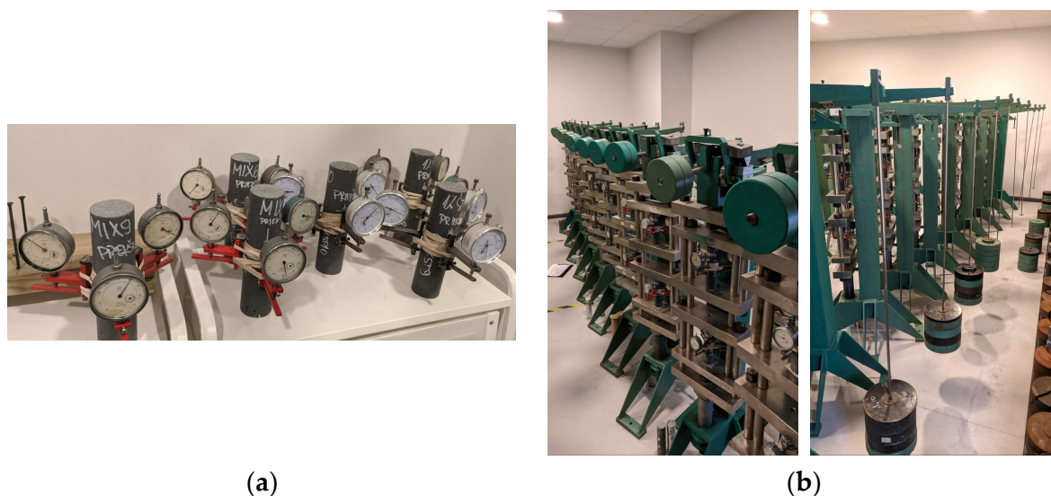
Figure 3. Plain and reinforced geopolymer specimens were used for shrinkage (a) and creep (b) testing.
