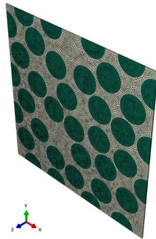
Figure 3. A 3D unit cell model with 37 fibers: green mesh denotes fiber and white is resin.
