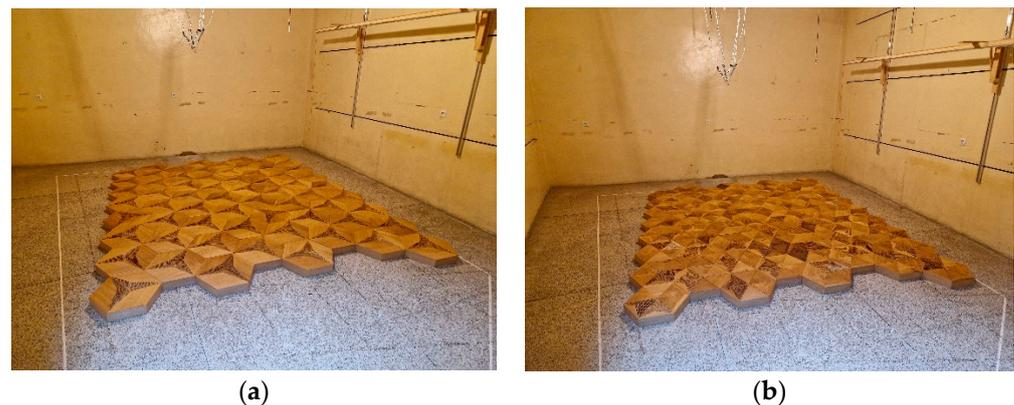
**Figure 10.** Photographs of the measured sequences in a reverberation chamber: (a) sequence with 100% perforated panels (CM-D); (b) sequence with 33% perforated panels (P-A) and 66% non-perforated panels.
