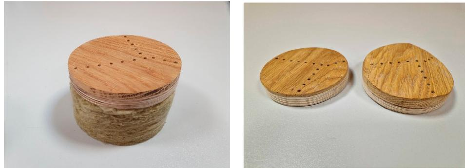
**Figure 2.** Test samples used in the impedance tube measurements.
