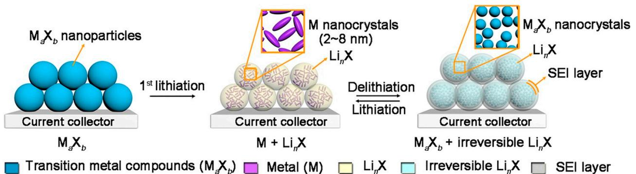
**Figure 11.** A depiction of the gradual growth of non-usable  $Li_nX$  when  $M_aX_b$  particles are used in anode LIBs. Provided by Lu et al. [151], Copyright 2018, with permission of Elsevier.
