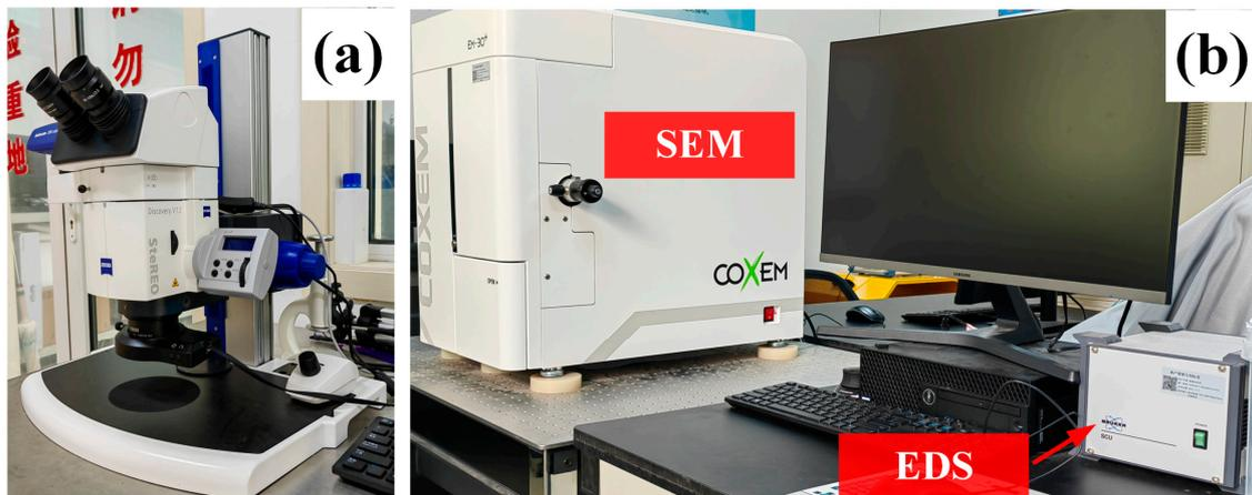
**Figure 4.** Fracture analysis system: (a) optical microscope (OM); (b) scanning electron microscope (SEM) and energy dispersive spectrometer (EDS).
