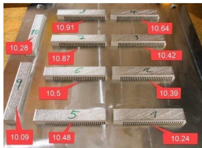
Figure 7. Placement of the test specimens on the build plate and their deformations.
