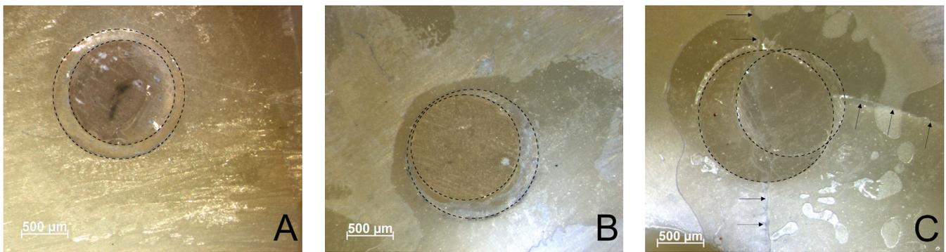
**Figure 1.** Showcase pictures of the plunger positions central (A), margin (B) and overlapping (C). Cavity circumference is marked by the large, dotted circle, plunger indentation by the smaller, dotted circle. Arrows indicate the visible fracture line within dentin.
