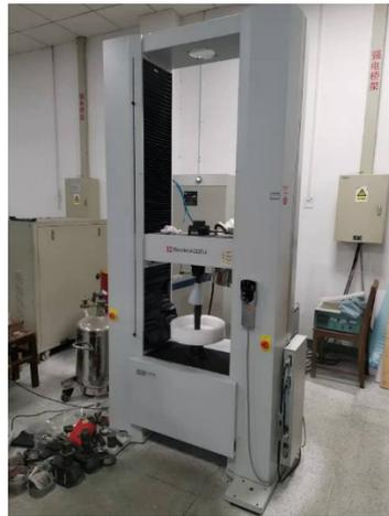
**Figure 9.** AG-IC 100 kN electronic universal testing machine.
