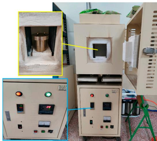
**Figure 2.** Exterior of high-temperature furnace and program controller.
