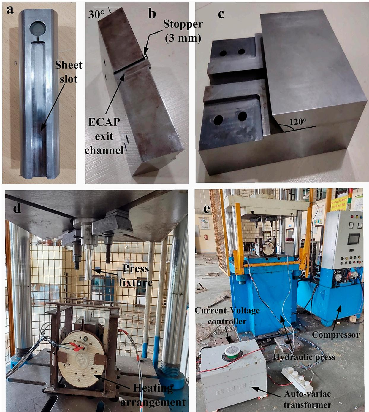
**Figure 4.** (a) Plunger with slot for Mg-RZ5 sheet; (b) Smaller unit having the exit point of the channel; (c) Larger unit having the 120° channel; (d) Experimental die setup along with its conductive heating arrangement; and (e) Hydraulic press machinery for ECAP accomplishment [13].
