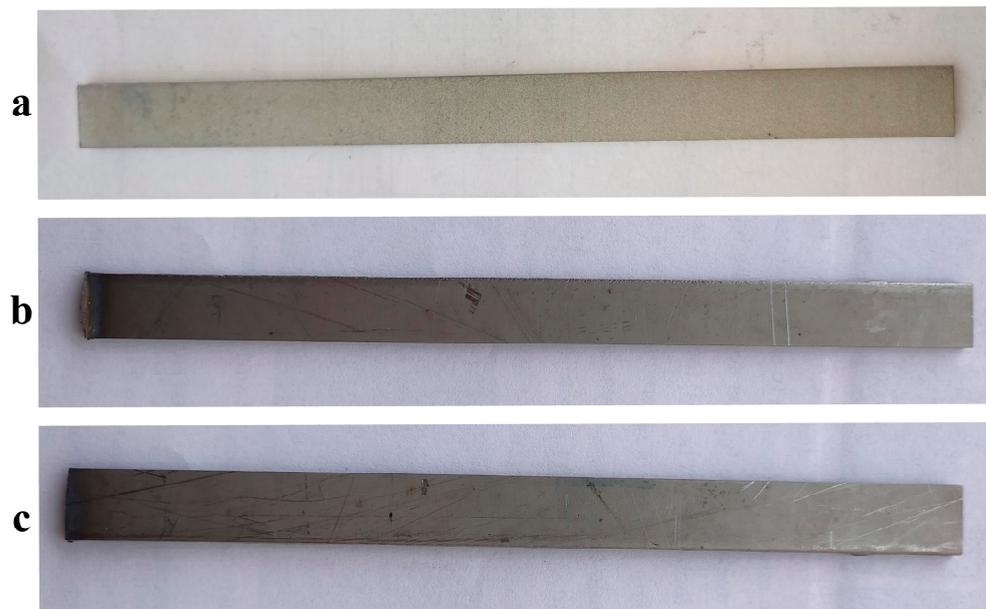
**Figure 5.** Magnesium RZ5 alloy sheet samples (a) before ECAP, (b) after ECAP two passes, and (c) after ECAP four passes.
