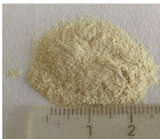
**Figure 9.** ZnO with the highest Zn content (from Experiment N° 10).
