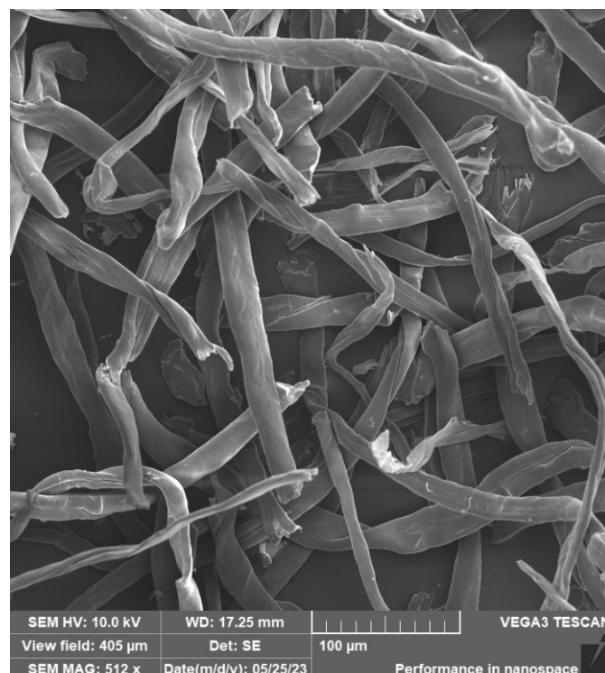
Figure 15. SEM of cotton fibre/flakes.
