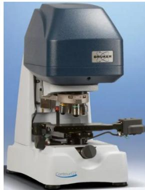
**Figure 5.** Three-dimensional topography profiler.
