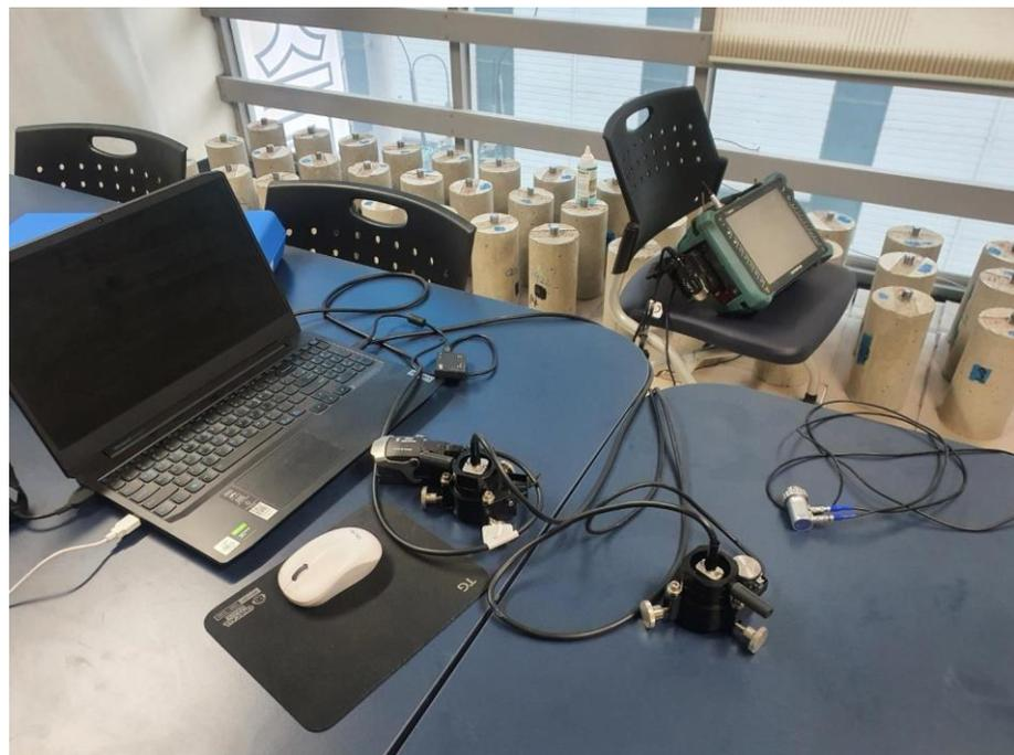
**Figure 6.** Testing equipment for PAUT.
