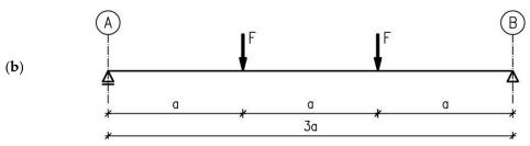
Figure 7. View of the test stand with the component under test (a) and static scheme (b).
