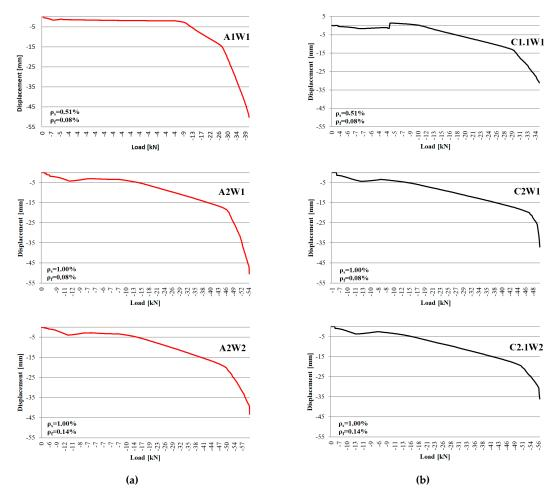
**Figure 14.** Load vs. displacement in beams during adhesive curing and failure loading, **(a,b)**—heated and non-heated beams with the same reinforcement ratios.
