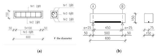
**Figure 1.** Details of tested elements–steel reinforcement (a) [32]; Method of strengthening of elements (b).
