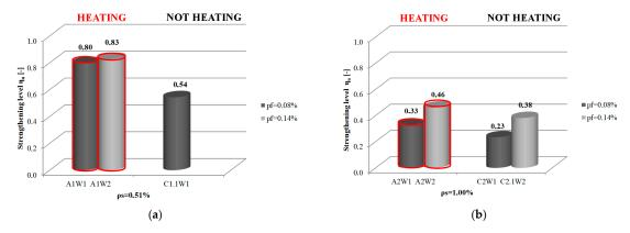
**Figure 13.** Graphical representation of the strengthening level of RC beams: (a) Beams with low steel reinforcement ratios; (b) Beams with high steel reinforcement ratios—red colour indicates the beams strengthened with heating of composite strip.
