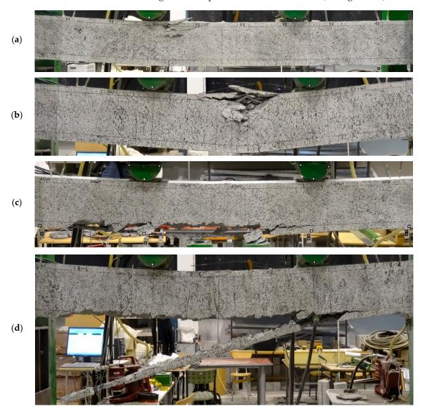
**Figure 11.** Failure modes of RC beams (examples): (a) Non-strengthened beam; (b) C2.1W2 beam; (c) A1W1 beam; (d) C1W2 beam.
