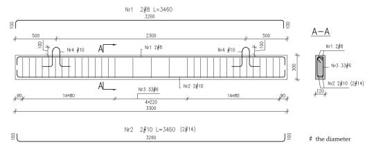
Figure 8. Details of two series of tested beams—steel reinforcement.
