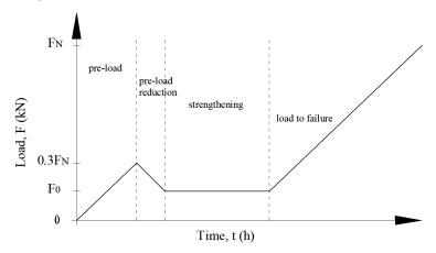
Figure 9. Loading program for beams strengthened with CFRP strips [33].
