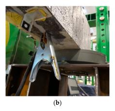
**Figure 10.** The process of strengthening reinforced concrete beams: (a) Making a groove from the bottom surface of the beams; (b) View of the copper flat bar with the current wire connected [33].
