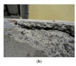
**Figure 5.** RC element failure: (a) underside of series 2 element; (b) partial sliding out of the strip from the copper flat bar clip, together with its debonding from the concrete cover (underside of the reinforced element).
