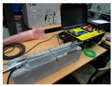
Figure 2. View of reinforced concrete element with attached prototype heating device.
