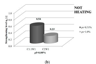
**Figure 12.** Relationship between strengthening effectiveness and steel reinforcement ratio: (a) Beams subjected to an accelerated strengthening process; (b) Beams in which the adhesive hardening process took 7 days.
