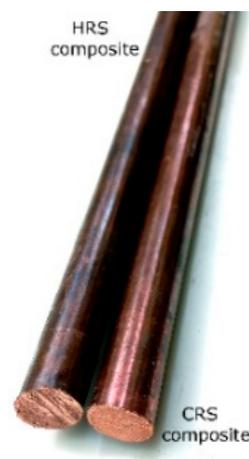
**Figure 1.** Bars of swaged Cu + Al<sub>2</sub>O<sub>3</sub> composite.
