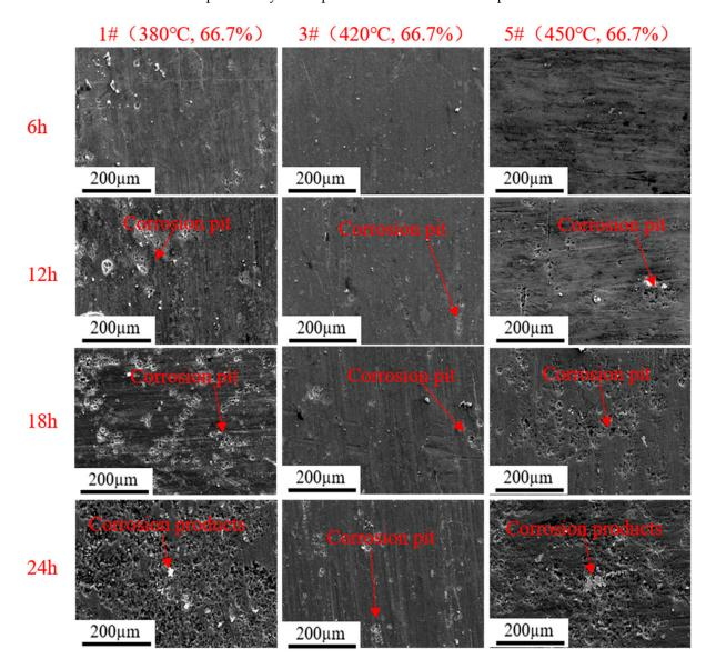
**Figure 11.** Corrosion morphology of the rolled AA7050 aluminum alloy immersed in 3.5 wt.% NaCl solution for 6, 12, 18, and 24 h (the samples were rolled with the same reduction at different temperatures).
