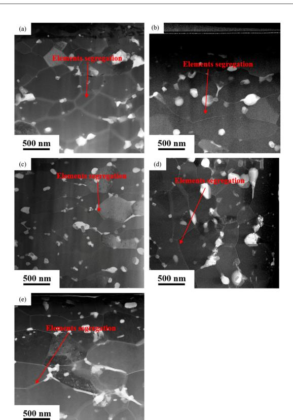
**Figure 2.** The HAADF micrographs showing the top regions of the near-surface deformed layers on hot rolled AA7050 aluminum alloy under different hot rolling conditions: (**a**) 1# (380 °C, 66.7%); (**b**) 2# (420 °C, 83.3%); (**c**) 3# (420 °C, 66.7%); (**d**) 4# (420 °C, 50%); (**e**) 5# (450 °C, 66.7%).
