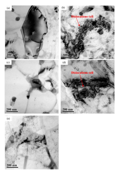
**Figure 7.** TEM micrographs showing the top regions of the near-surface deformed layers on hot rolled AA7050 aluminum alloy under different hot rolling conditions: (**a**) 1# (380 °C, 66.7%); (**b**) 2# (420 °C, 83.3%); (**c**) 3# (420 °C, 66.7%); (**d**) 4# (420 °C, 50%); (**e**) 5# (450 °C, 66.7%).
