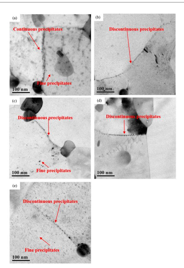
**Figure 6.** TEM micrographs showing the top regions of the near-surface deformed layers on hot rolled AA7050 aluminum alloy under different hot rolling conditions: (a) 1# (380 °C, 66.7%); (b) 2# (420 °C, 83.3%); (c) 3# (420 °C, 66.7%); (d) 4# (420 °C, 50%); (e) 5# (450 °C, 66.7%).
