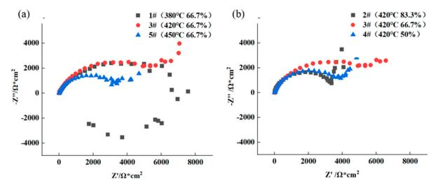
**Figure 10.** Nyquist diagrams of hot rolled AA7050 aluminum alloy in 3.5 wt.% NaCl solution: (**a**) the alloy samples rolled with the same rolling reduction, at different rolling temperature; (**b**) the alloy samples rolled at the same hot rolling temperature, with different rolling reduction.
