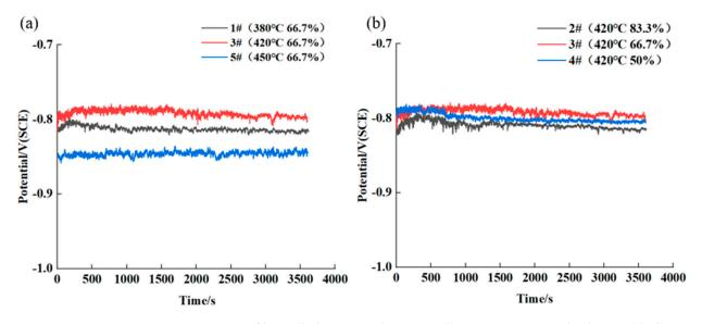
**Figure 8.** OCP of hot rolled AA7050 aluminum alloy in 3.5 wt.% NaCl solution: (**a**) alloy samples rolled with the same rolling reduction, at different rolling temperature; (**b**) alloy samples rolled at the same hot rolling temperature, with different rolling reduction.
