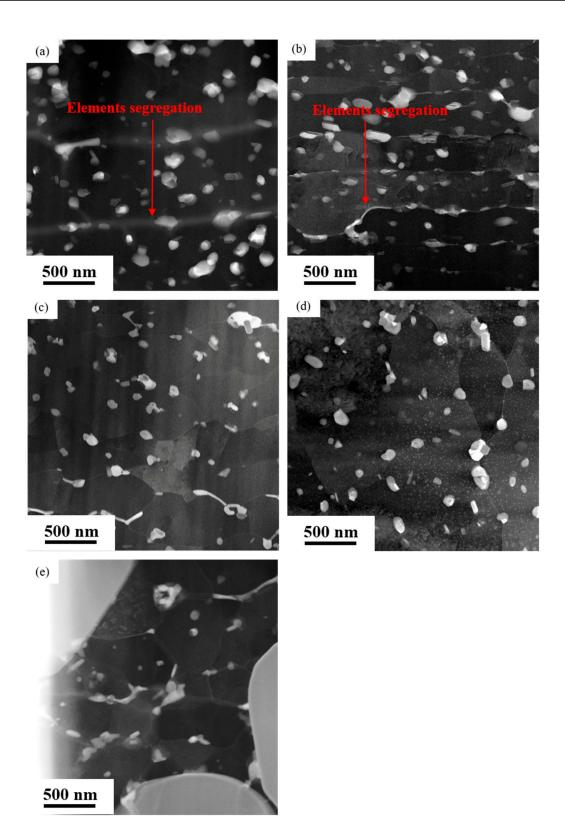
**Figure 3.** The STEM-HAADF micrographs showing the bottom regions of the near-surface deformed layers on hot rolled AA7050 aluminum alloy under different hot rolling conditions: (**a**) 1# (380 °C, 66.7%); (**b**) 2# (420 °C, 83.3%); (**c**) 3# (420 °C, 66.7%); (**d**) 4# (420 °C, 50%); (**e**) 5# (450 °C, 66.7%).
