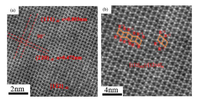
**Figure 5.** (**a**) The lattice image of the rounded plate precipitate along [112] <sub>Al</sub> axis; (**b**) the enlarged image in (**a**).
