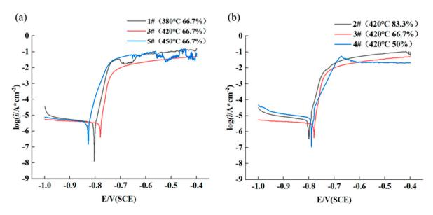
**Figure 9.** Potentiodynamic polarization curves of hot rolled AA7050 aluminum alloy in 3.5 wt.% NaCl solution: (**a**) the alloy samples rolled with the same rolling reduction, at different hot rolling temperature; (**b**) the alloy samples rolled at the same hot rolling temperature, with different rolling reduction.
