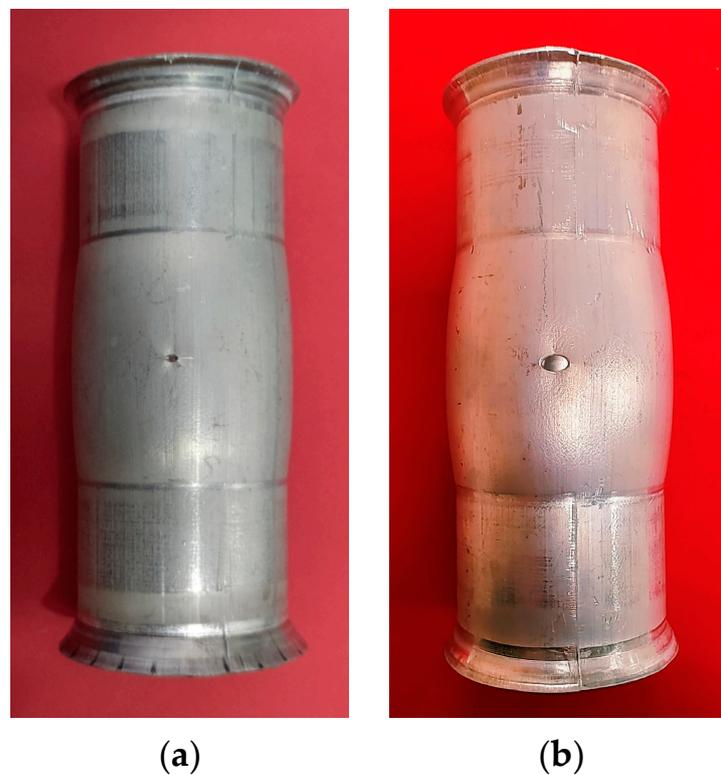
Figure 20. Tubular specimens after HB experiments with initial apertures of: (a) 2 mm, and (b) 4 mm.
