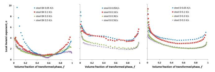
**Figure 7.** The Local Avrami exponent *n* for low cooling rates as a function of volume fraction of transformed phase *f* for steels BX, B and D.
