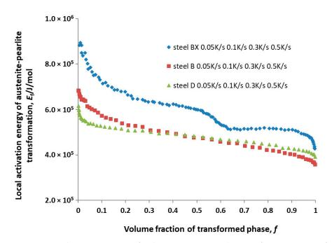
**Figure 6.** Local activation energy for the austenite-to-pearlite transformation  $E_f$  as a function on the volume fraction of transformed phase *f* calculated in [8,10–13].
