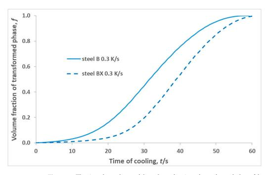
**Figure 11.** The time dependence of the volume fraction of transformed phase *f* for steels BX and B, subjected to continuous cooling at a rate of 0.3 K/s.
