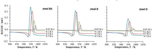
The time derivatives on the dilatometry signal  $\left(\frac{d\Delta L}{dt} - T\right)$  versus the temperature for steels BX, B and D at all cooling rates used are shown in Figure 10.
