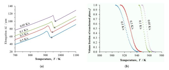
**Figure 4.** Dilatometric study of steel B continuously cooled at cooling rates  $\beta = 0.05$  K/s, 0.1 K/s, 0.3 K/s and 0.5 K/s: (**a**) temperature dependence of changes to the length of the dilatometric sample,  $\Delta L$ ; triangles mark the onset of phase transformation; (**b**) temperature dependence of the transformed volume fraction *f*.
