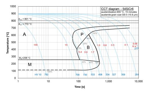
Figure 8. CCT diagram of steel BX.
