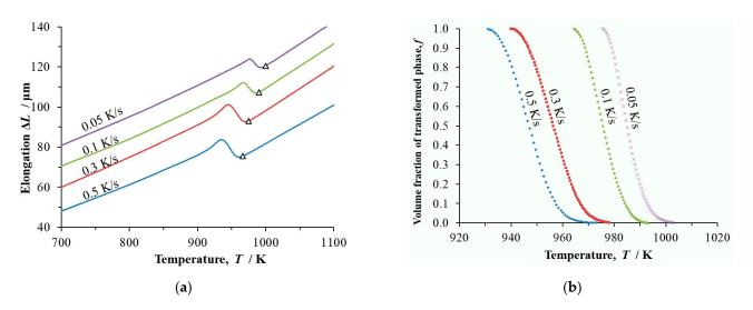
**Figure 5.** Dilatometric study of steel D continuously cooled at cooling rates  $\beta = 0.05$  K/s, 0.1 K/s, 0.3 K/s and 0.5 K/s: (**a**) temperature dependence of changes to the length of the dilatometric sample,  $\Delta L$ ; triangles mark the onset of phase transformation; (**b**) temperature dependence of the transformed volume fraction *f*.
