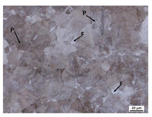
**Figure 1.** Optical metallography of the microstructure of steel BX after the completion of continuous cooling at a cooling rate of 0.05 K/s (F = Ferrite, P = Pearlite).
