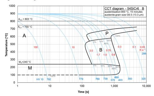
Figure 9. CCT diagram of steel B.
