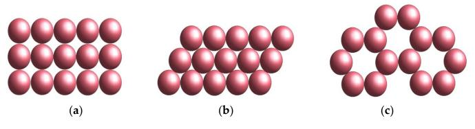
**Figure 1.** Planar packing of spheres in the case of: (**a**) Square packing; (**b**) Hexagonal packing; (**c**) Basic hexagonal structure with missing spheres.
