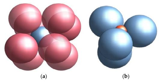
**Figure 3.** (a) Packing of small spheres in between big ones in a cubic arrangement; (b) Packing of small spheres into cells with tetragonal lattice.
