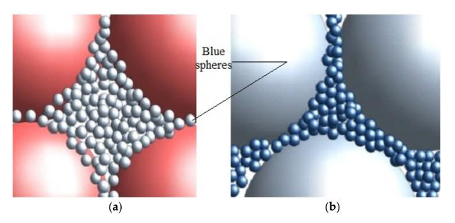
**Figure 4.** (a) Scheme of big spheres with a diameter  $d_1$  with a space in-between filled up with spheres of  $D_2 = K$ , diameter; (b) Smaller spheres with a diameter  $D_3 = K^2$  filling up the space in-between the spheres of a diameter  $D_2$ . The free space filling could be continued till the packing of the smaller spheres reaches the diameter  $D_n = K^{n-1}$ .
