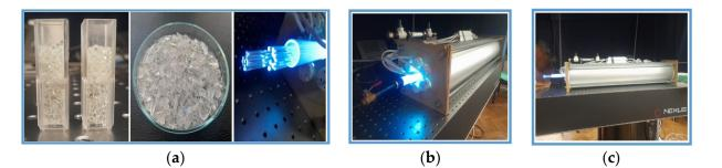
**Figure 6.** Decontamination core filled up with metamaterials. (**a**) Quartz spheres (**left**), crushed grains quartz (**center**) and fibre fragments (**right**); (**b**) The core submitted to irradiation; (**c**) Al cylinder for protection and loss minimization.
