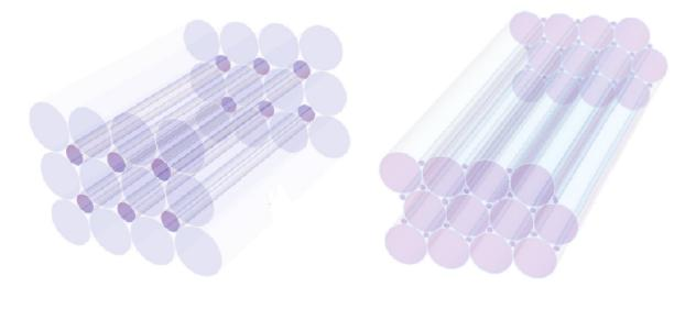
Figure 5. (a) Packing schemes with square; (b) hexagonal fibres fragments, respectively.
