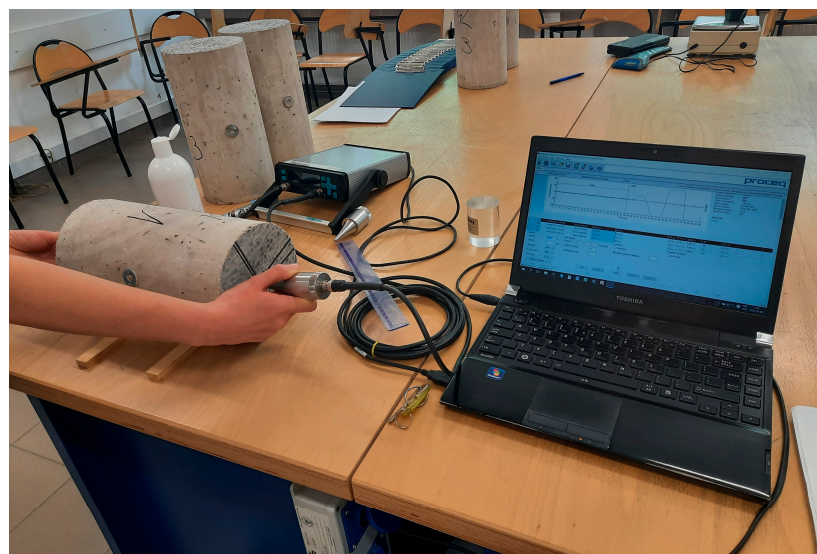
Figure 5. A concrete specimen with the measuring apparatus for determination of dynamic modulus of elasticity according to ultrasonic pulse velocity method.
