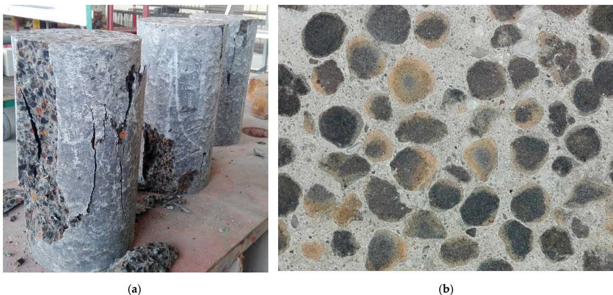
Figure 6. Specimens of lightweight concrete after compressive strength test: (a) General view; (b) Fracture form.
