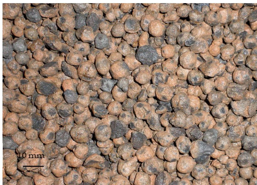
Figure 1. Sintered fly ash aggregate 4/8 mm (Lytag) used for concretes preparation.
