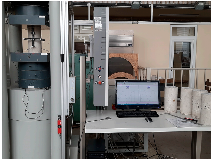
Figure 4. A concrete specimen with the measuring apparatus for determination of secant modulus of elasticity according to EN 12390-13.
