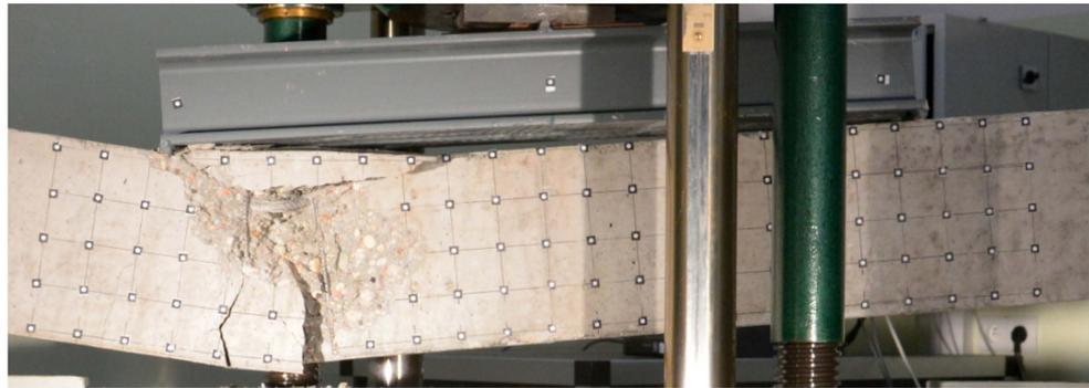
Figure 9. Compressive zone failure in beam No. 2.
