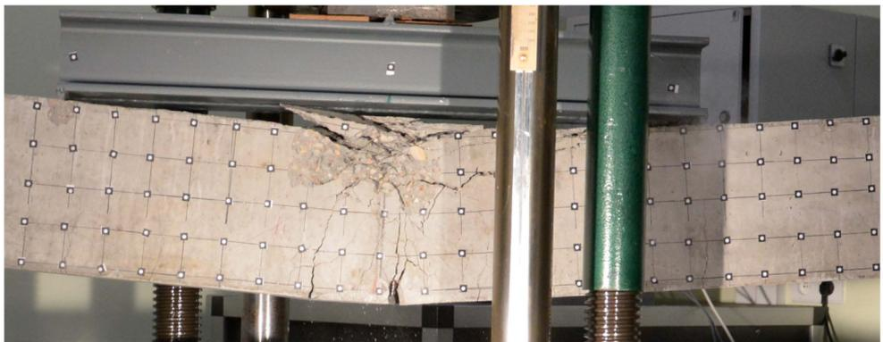
Figure 8. Compressive zone failure in beam No. 1.
