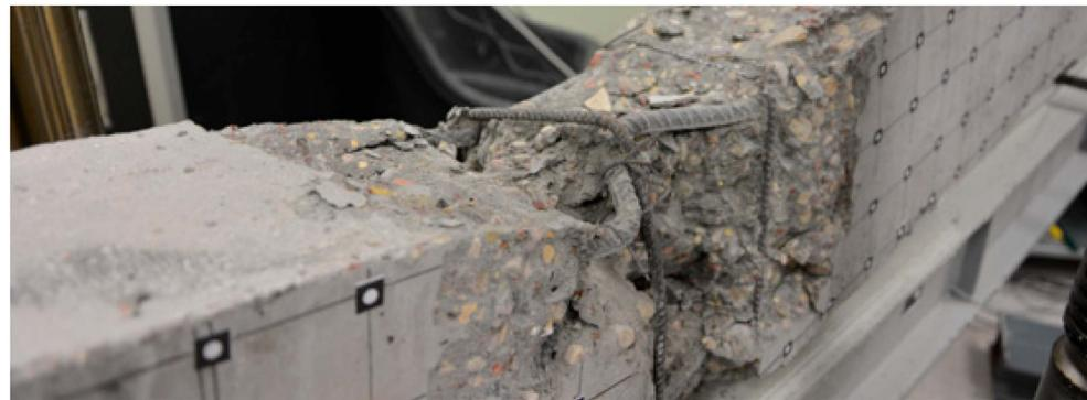
Figure 10. Local buckling of the steel reinforcing bars in beam No. 1.
