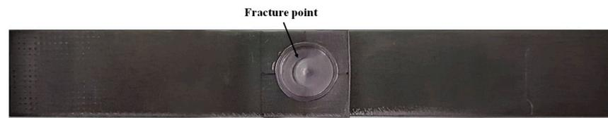
**Figure 9.** Fractured specimen after lap-shear test.
