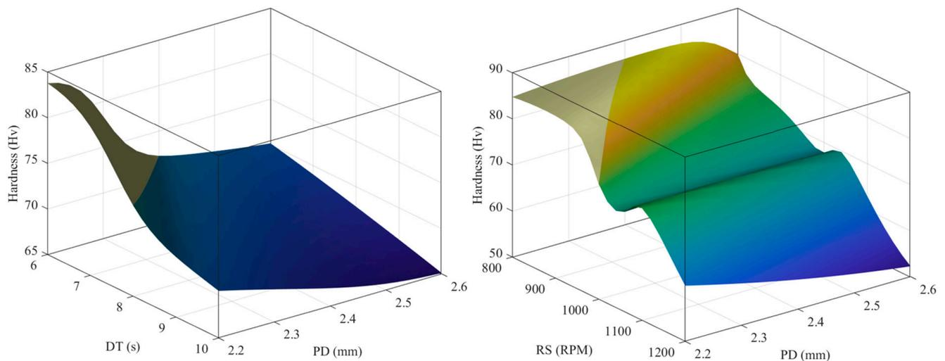
**Figure 12.** Predicted surface to hardness target based on design parameters.
