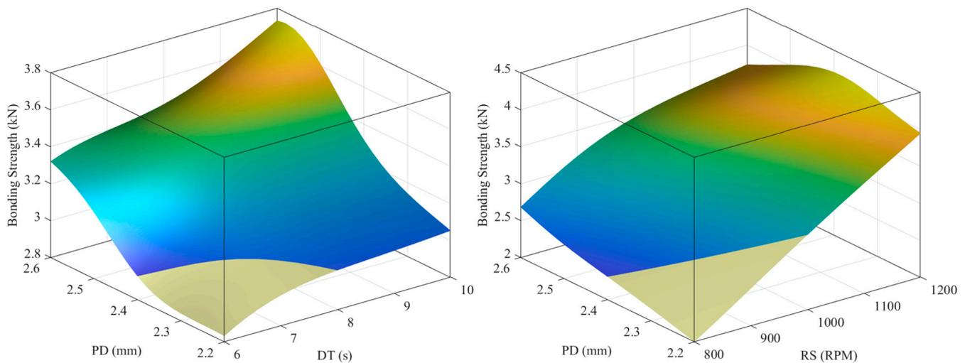
**Figure 13.** Predicted surface to bonding strength target based on design parameters.
