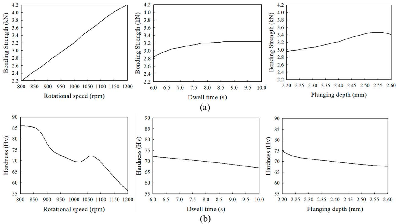
Figure 14. Variation of the objective functions (a) bonding strength and (b) hardness for each parameter when the other process parameters are held fixed.
