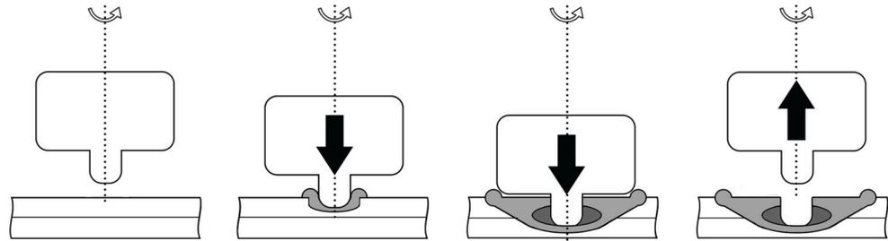
**Figure 1.** Schematic of the friction stir spot welding (FSSW) procedure.
