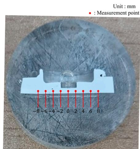
Figure 8. Measurement points for weld zone.
