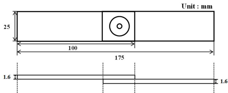
Figure 5. Typical specimen for lap-shear test.
