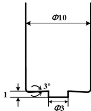
Figure 4. FSSW tool geometry.
