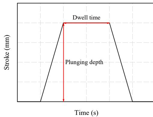
Figure 3. Stroke profile in the FSSW process.
