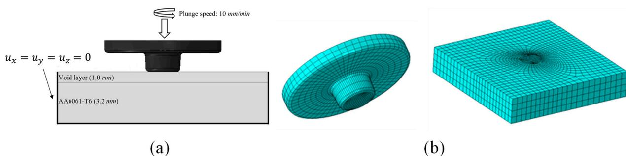
**Figure 6.** Schematic finite element (FE) model: (a) Boundary conditions of the FE model (b) Mesh of FE model.
