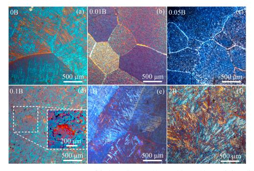
with a high boron content of 1–2%, the average grain size was 710  $\pm$  50  $\mu$ m, i.e., the value was similar to the boron–free alloy.
