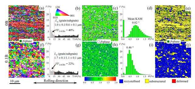
**Figure 7.** (**a**,**f**) EBSD-IPF maps, (**b**,**g**) grain boundary misorientation angle distributions, (**c**,**h**) kernel average misorientation (KAM) maps, (**d**,**i**) local misorientation distributions and (**e**,**j**) recrystallized fraction map of the (**a**–**e**) 0B and (**f**–**j**) 0.1B alloys after annealing for 30 min at 875 °C.
