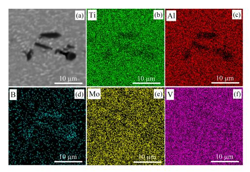
Figure 4. (a) SEM images and (b–f) EDS SEM maps of the hot-rolled 0.1B alloy.
