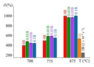
**Figure 9.** Elongation to failure ( $\delta$ ) dependency in a temperature range of 700–875 °C of the investigated alloys.
