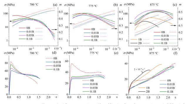
**Figure 8.** (**a**–**c**) Stress vs. strain rate (dotted lines) and *m* value vs. strain rate (solid lines) obtained by a step-by-step decrease in the strain rate and (**d**–**f**) stress–strain curves at a constant strain rate of  $1 \times 10^{-3} \text{ s}^{-1}$  at (**a**,**d**) 700 °C, (**b**,**e**) 775 °C, and (**c**,**f**) 875 °C.
