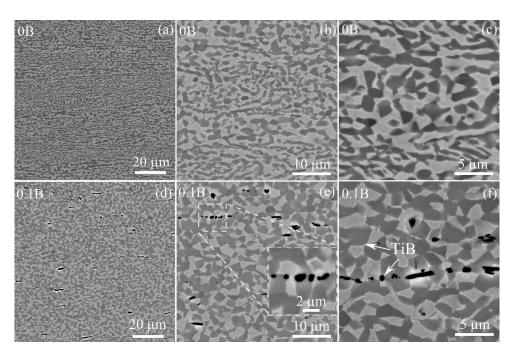
Figure 6. Microstructures of the (a-c) 0B and (d-f) 0.1B alloys after annealing for 30 min at 875 °C.
