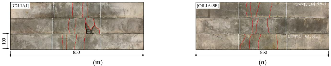
**Figure 8.** Crack patterns (the unit of length is mm): (a) NF-I; (b) C1L1A0; (c) C2L1A0; (d) C3L1A0; (e) C4L1A0; (f) C2L1A1; (g) C2L1A1SE; (h) C1L1A4SE; (i) C2L1A2; (j) C2L1A4SE; (k) C2L1A3; (l) C3L1A4SE; (m) C2L1A4; (n) C4L1A4SE.
