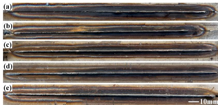
**Figure 2.** Schematic diagram of weld bottom at (a) 2 kW, (b) 2.2 kW, (c) 2.4 kW, (d) 2.6 kW, and (e) 2.8 kW.
