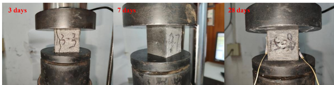
Figure 5. Uniaxial compressive strength test of 3 days, 7 days, and 28 days test block curing.
