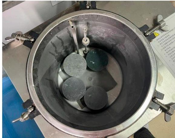
**Figure 2.** Specimens after vacuum saturation.
