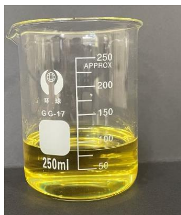
Figure 1. ADN-based liquid propellants at ambient temperature and pressure (A high-energy ionic liquid propellant).
