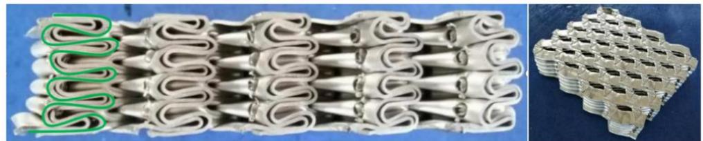
**Figure 16.** The final configuration of axial deformation.
